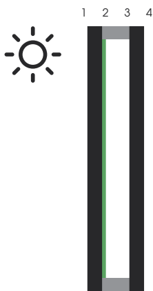
Coating on Position #2 Offers a slightly better solar performance than Low E on #3.
